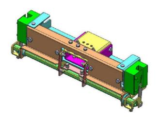
Safety gear for counterweight for installations on the slab (where underneath people have access)
