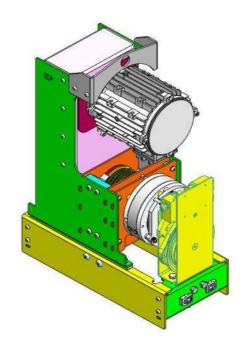
The traction unit is installed between the guides
