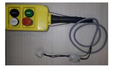
Keypad to be connected at the homelift for the installation and maintenance operations.
