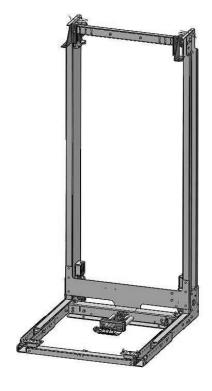
Cantilever sling with safety roping points inspectionable from the bottom of the cabin. Cabin wall removal is no longer required
